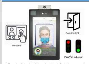
When the SpeedFACE reader is installed at a secured office entrance, visitors can intercom the receptionist for access. If entry is authorized, the receptionist may remotely unlock the door once the SpeedFACE reader has confirmed compliance with the body-temperature and face mask policies.
