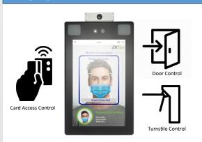
When the SpeedFACE reader is installed at employee entrances and connected to electronic access control system, it will provide a secondary means of verification. Employees will scan their door access card and then allow the SpeedFACE reader to verify compliance with body temperature and/or face mask policies. Once verified, the reader will pass the employees card data to the access control system for door unlocking.
